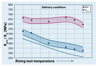
The anticipated and observed tensile and yield strength data are in all cases above the minimum levels required in EN 10028, Part 3, even at elevated temperatures.
