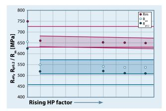
On a statistical view, 99% of all measured tensile strength data are present within the scatter band marked in red. Yield strength follows a similar pattern (blue scatter band). As the Hollomon parameters (HP) rise, the data decrease as expected, but the steel is designed such that the minima specified in the standard are never undercut.
