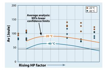
A significant improvement in Charpy V-notch toughness has been achieved for DILLINAL. Our customers can thus use this steel at low temperatures without difficulty thanks to its enhanced reserves of toughness.
