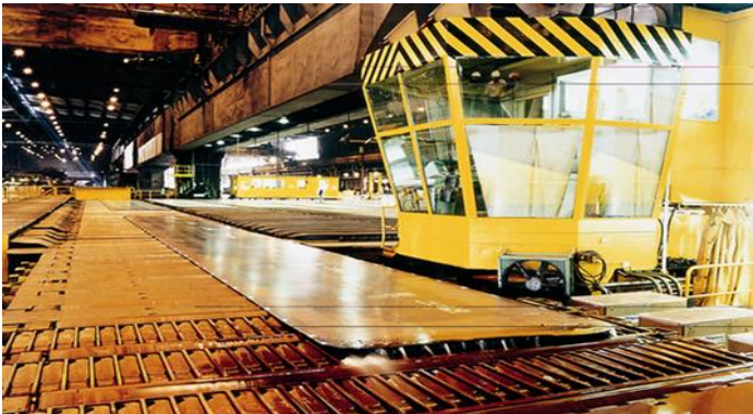
Ultrasonic heavy plate testing line for plate thicknesses up to 55 mm in the shear line
