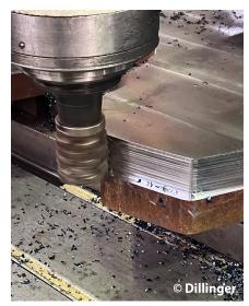
DILLIDUR steels are very well suited for machining in spite of their high strength and hardness. However, some basic rules must be observed when machining these hardened steels. Vibrations should be avoided. It is therefore advisable to work on a machine that is as rigid as possible and to keep the gap between the workpiece and the machine (support) to a minimum. Similarly, it is advisable to fix the workpiece firmly to the workbench.
