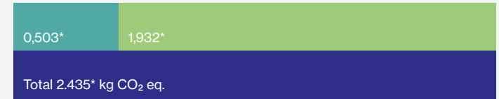
Heavy plate (Dillingen, Dunkerque) via BF/BOF
