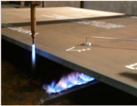
Preheating of DILLIMAX
