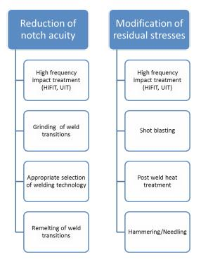
Potentials for improvement of the fatigue strength of weld details
