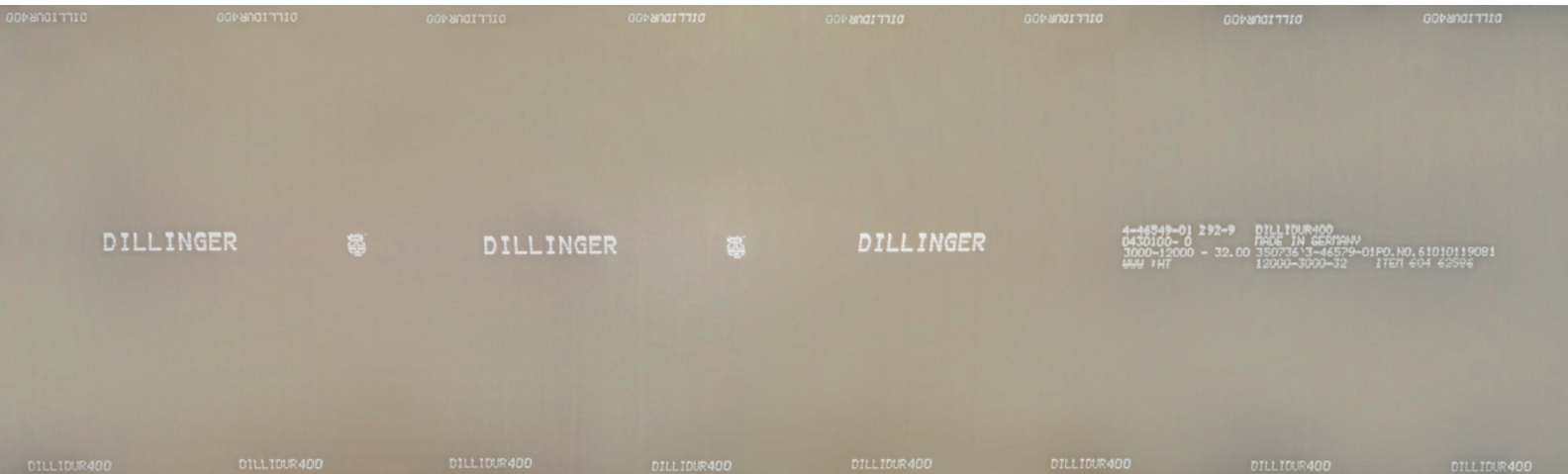
Primed plate (shop primer) with customized marking
