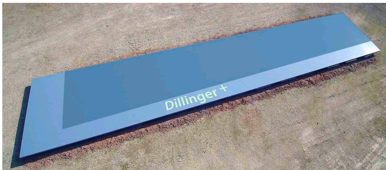
The world’s largest TM plate - a DI-MC 355 T
