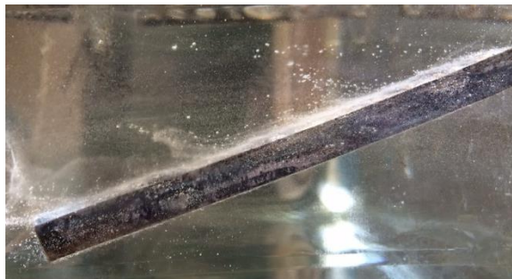
Figure 6: Diffusible hydrogen escapes from the test bead in the glycerin bath.
