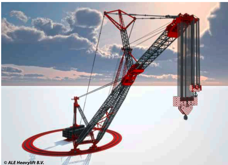
The fixed jib consisting of ultra-high-strength DILLIMAX steel serves as an extension of the boom and can, with its length of up to 120 m, lift a maximum of 3,400 tonnes.
