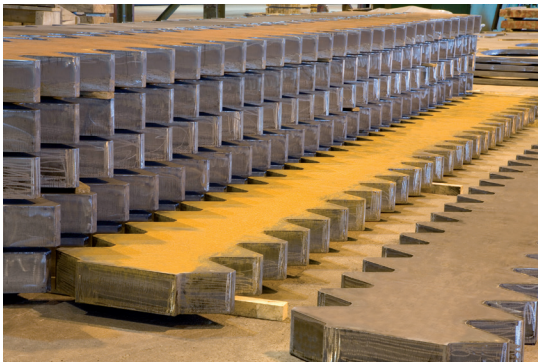
Flame cut gear racks in Dillinger Hütte's Heavy Fabrication shop
