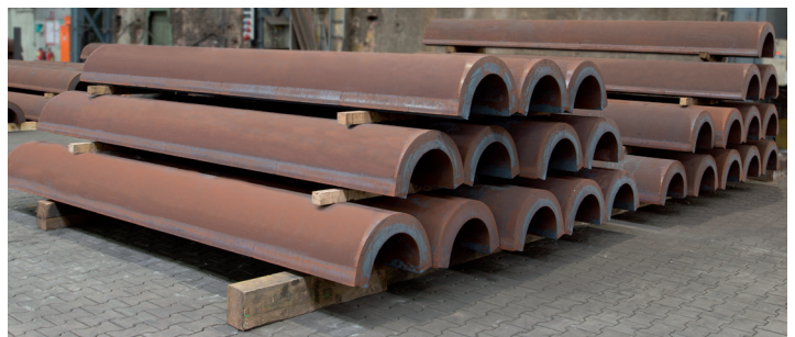
Hot-formed chords in Dillinger Hütte's Heavy Fabrication shop
