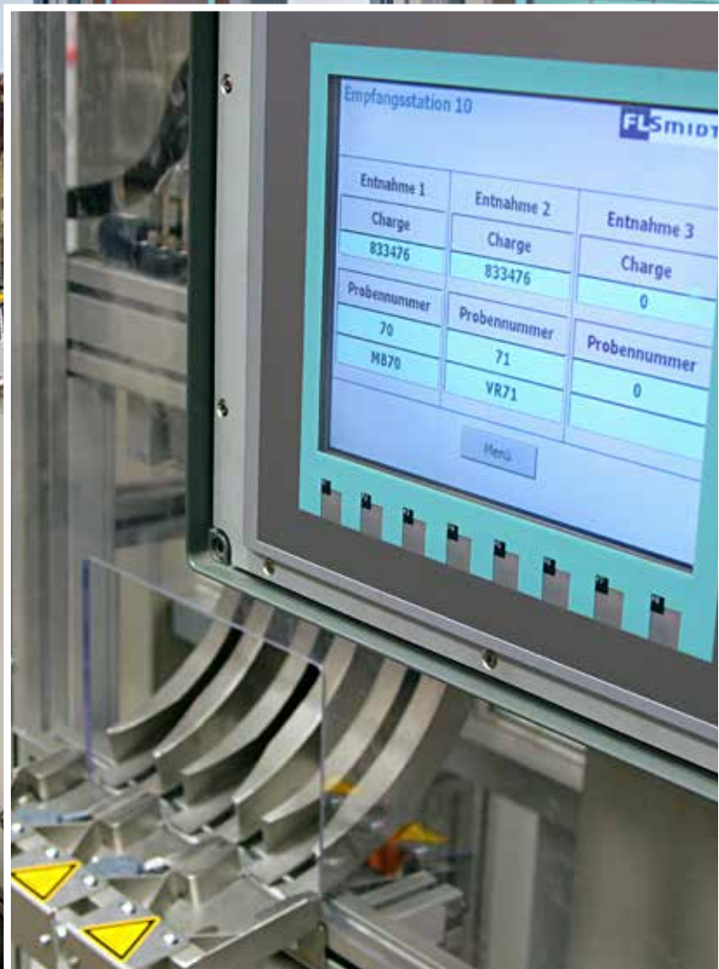
Analytical: The new pneumatic tube delivery system delivers around 126,000 samples per year to one of the 13 receiving stations in the new LD laboratory for further analysis.
