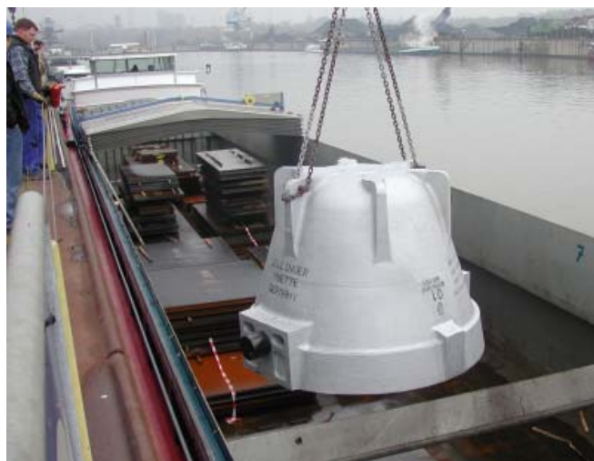
Slag pot (34 m 3 / 63 t) being loaded at the company's pier in DILLINGEN
