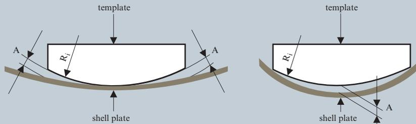
The shape deviations are measured as distance  $A$  between a template board (with a chord length of 500 mm respectively 2.000 mm) fitted with the radius and the plate curvature: the checking is carried out as shown in the adjacent sketch after the plates are laid down on a measuring bed set to the nominal radius.
