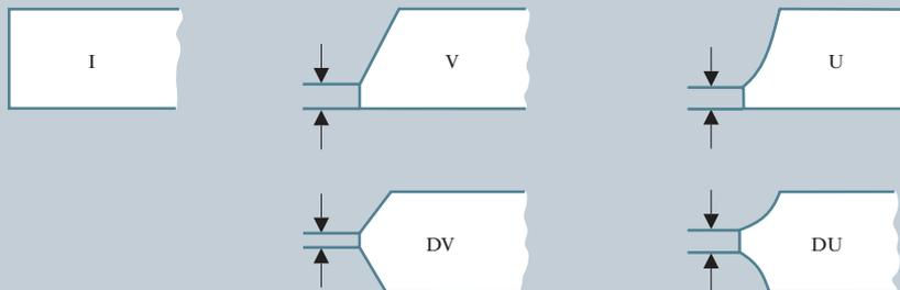
Notes: details of weld-edge preparation e.g. root radius and slope angle must be agreed.
