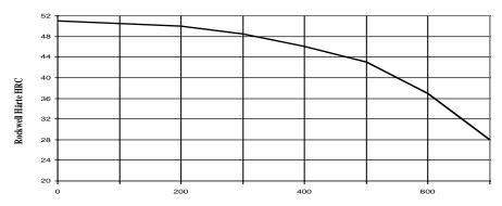
Tempering temperature [°C] (valid for soaking time 1 h, air cooling)
