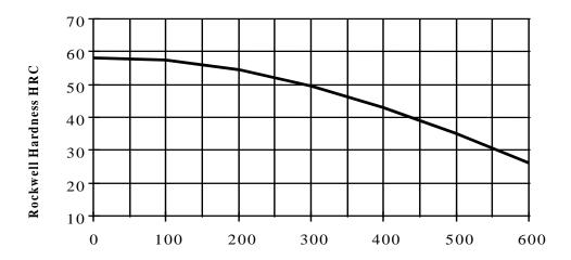
Tempering temperature [°C] (valid for soaking time 1 h, air cooling)
